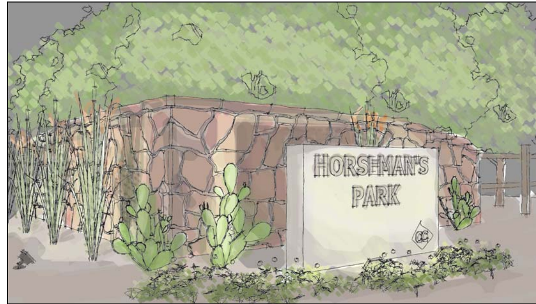
Illustration of possible Horseman's Park entry. A high rock wall protects horses from vehicle headlights at night. Contrasting materials help announce the visitor's arrival to Horseman's Park.
