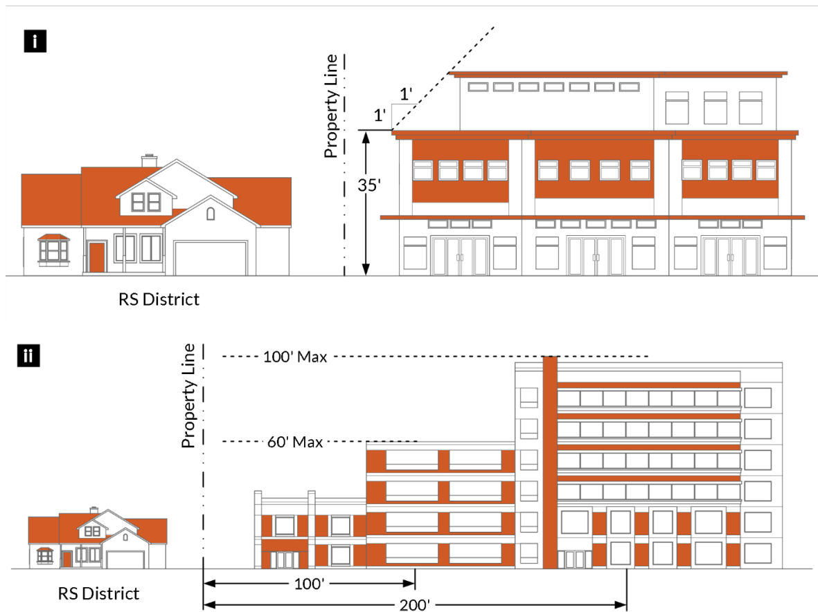
Figure 30.04-18: Residential Adjacency – Height Step Backs and Limits
